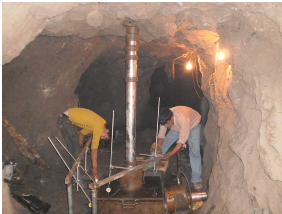
Photograph 4: A View of Direct Shear Test About to be Started- Ratle H.E. Project, J&K
