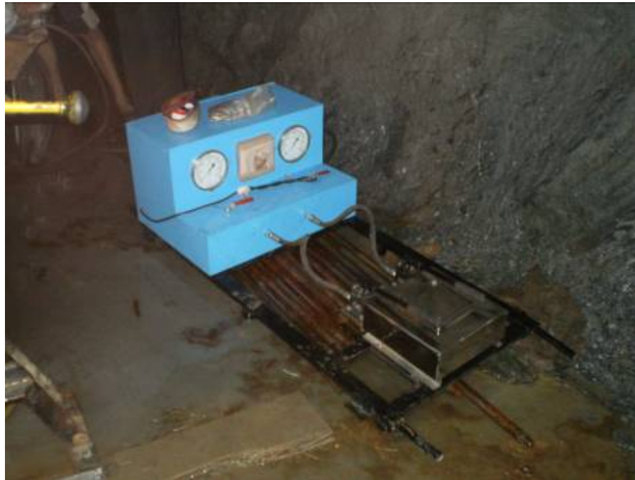
Fig. 5 (a): Hydraulic Fracturing Equipment Used
