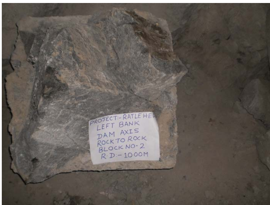
Photograph 5: A View of the Overturned Block After Shear Test (Rock to Rock)- Ratle H.E. Project, J&K
