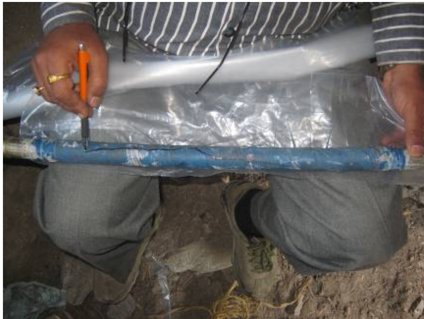
Fig. 9: Hydraulic Fracturing Test-Examining and Tracing Fracture Impression
