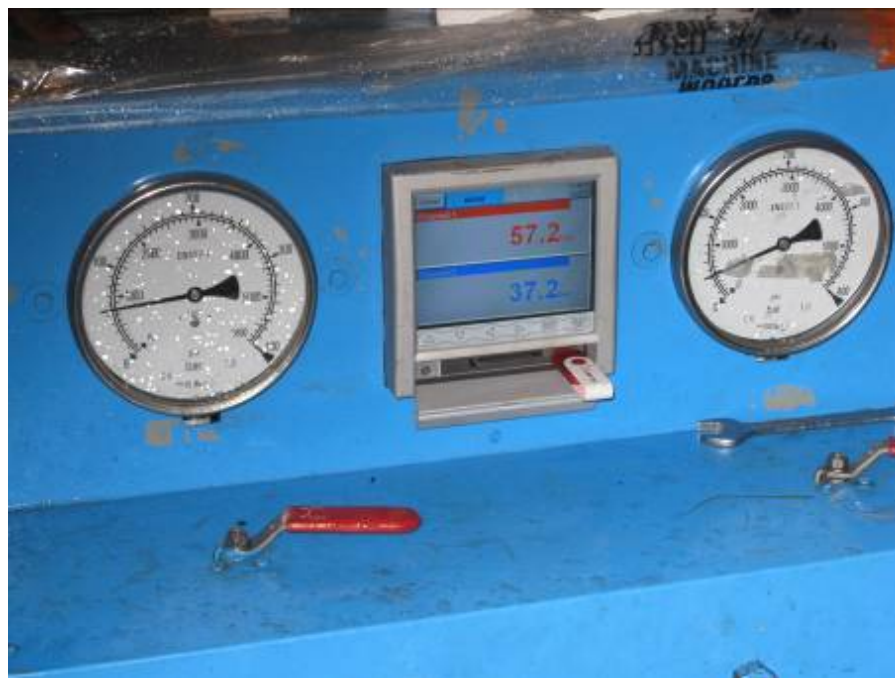
Fig. 5 (b): A Close up of Monitoring System of Hydraulic Fracturing Equipment
