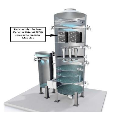
Figure 5: SPC Based FGD System
